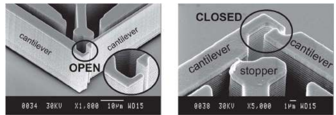
Fig. 8. Closeup view SEM pictures of the hook mechanism: (a) unlocked state (open switch), (b) locked state (closed switch).
