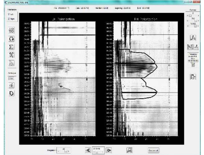
Fig. A.1. Screen capture of the catalog construction software. The LH and RH dynamic spectra for the whole observation of 20/08/2010 are shown. The frequency scale is horizontal (10 to 40 MHz) and the timescale is vertical, increasing upward. This observation lasted for 8 h with a calibration sequence visible every hour. An emission is visible with dominant RH polarization, surrounded by a polygonal contour drawn by hand (with the mouse). The contour was drawn in 4 parts to exclude the calibration sequences of the computed average intensities. The various buttons and tools around the dynamic spectra serve for the interactive display, contour drawing, emission type selection, and recording.
