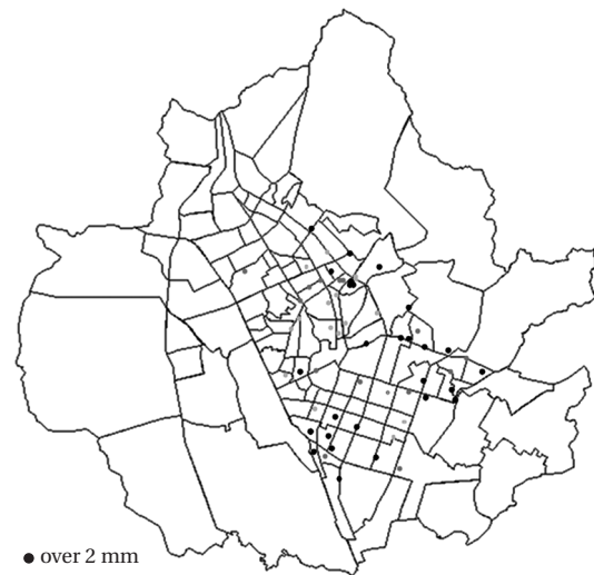
Fig. 16. Location where corrosion depth will exceed 2 mm by 2030.
