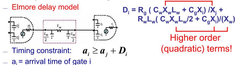
Delay model and timing constraint used in previous work in DAC 2005:  $a_i \ge a_i + d_i^0 + d_i$  linear terms!
