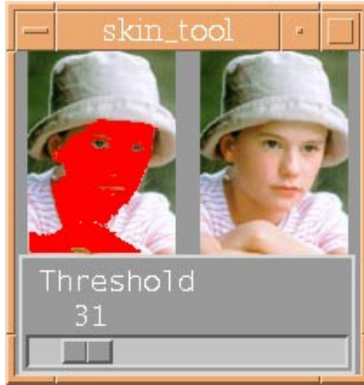
Figure 10: Snap shot of the tool for segmenting the skin region of an image. The left image shows the completed manual segmentation with the skin pixels highlighted in red. The right image shows the original image.
