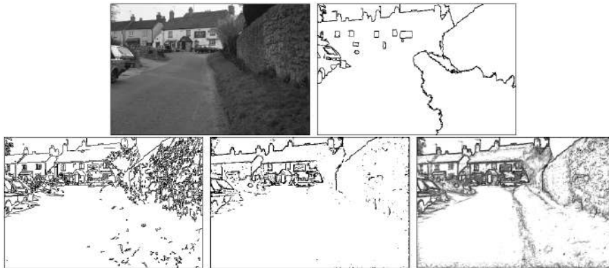
Fig. 1. A typical Sowerby image (top left panel) with its ground truth segmentation (top right panel), and its segmentation using the Canny edge detector (bottom left panel) and by statistical edge detection (bottom center panel). Statistical edge detection has fewer false negatives in the textured regions and is also better at detecting edges which are partially defined by texture. By contrast, the Canny detector is slightly better at precision of certain edges. The log-likelihood ratios are also shown (bottom right panel).
