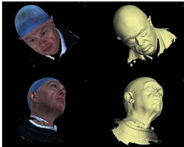
Fig. 3 Headspace dataset example. Left: texture mapped mesh rendered from two viewpoints. Right: monochrome mesh rendered from the same two viewpoints
