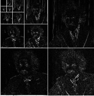
Figure 2. Coefficient magnitudes of a wavelet decomposition. Shown are absolute values of subband coefficients at three scales, and three orientations of a separable wavelet decomposition of the “Einstein” image.
