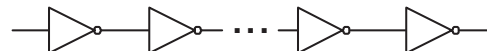
Fig. 1: Circuit with linear structure has timing complexity O[N^2] since no small local sensitivity terms can be lumped
