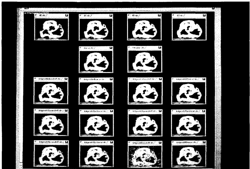
Figure 3: Slices computed from CT data. Interpolation techniques were used to create a new slice between original slices 32 and 33. Window titles depict the type of interpolation used.
