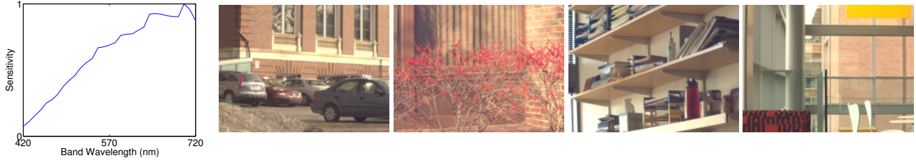
Figure 1. Hyperspectral Database of “real-world” images. Each image has a spatial resolution of 1392 \times 1040 with thirty-one spectral measurements at each pixel. Left: Camera sensitivity for each wavelength band. Right: Typical images of indoor and outdoor scenes from the database, rendered in sRGB.
