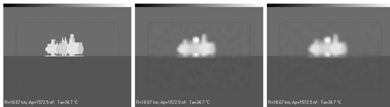
Figure 5: False color representation of a target after processing: refraction only (left), refraction, blur and noise (middle), and refraction, blur, noise and digitization. ( Projected data in the bottom are not representative for the presented synthetic target. )
