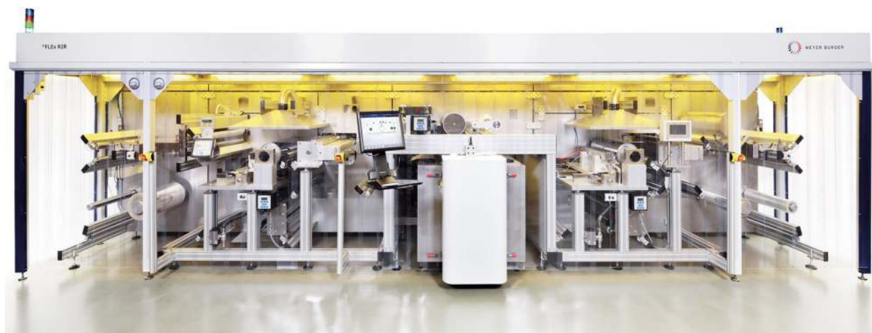
Fig. 15. Scale up for thermal ALD to very large area has been done, for instance, by thermal spatial ALD concepts for roll-to-roll coating such as Meyer Burger's FLEx R2R sALD tool. Such concepts should be extendable to plasma ALD, for instance, by including an atmospheric SDBD plasma as shown in Fig. 6. Picture courtesy of Meyer Burger (Ref. 217).
