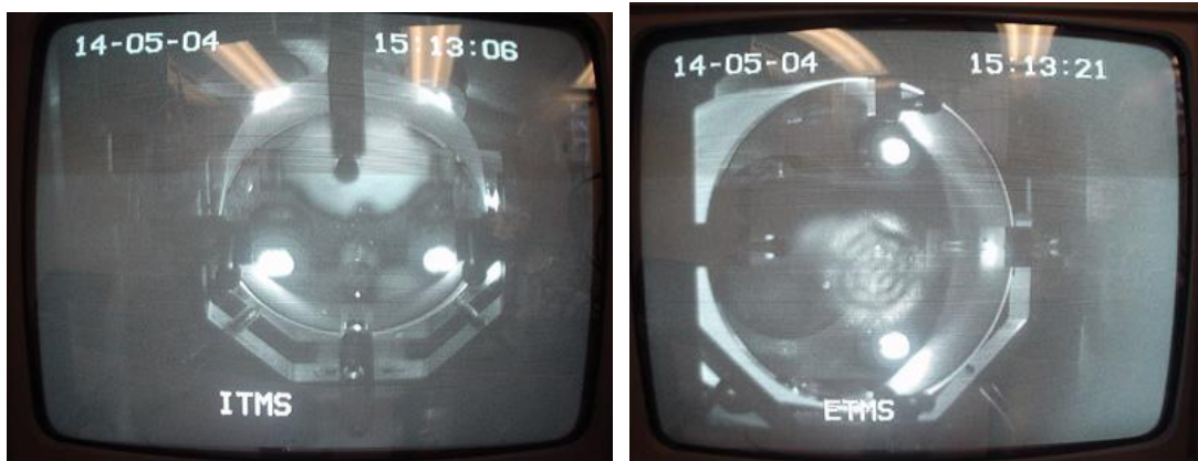
Figure 11: The pictures show the images from the CCD cameras mounted outside the vacuum tanks. The cameras are used to monitor the test masses during locking and operation. At the south end test mass (ETMS) we can see the higher order modes oscillating inside the 80m cavity.
