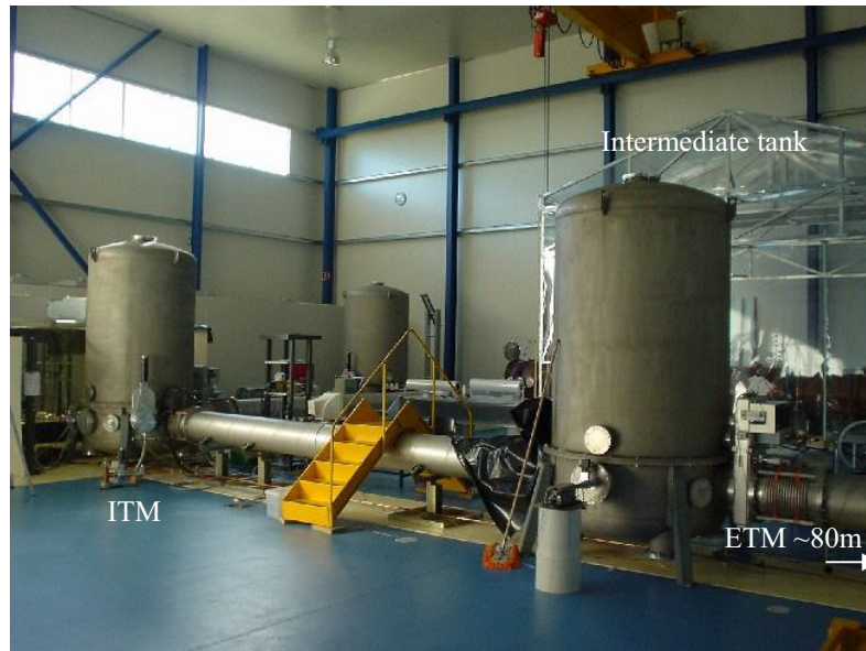
Figure 8: View of the main lab, where it is possible to see the ITM vacuum tank and the intermediate tank, where the ITM will be installed for Gingin test 3. At the actual ITM tank we will mount the power recycling mirror.
