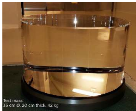
Figure 6. Advanced Virgo test mass. The Fused Silica substrate 0.35 m diameter is 0.2 m thick, for a total weight of 42 kg.
