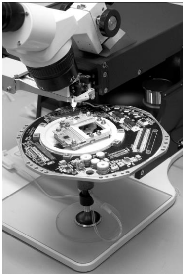
Figure 9. The top photo shows seven qualification-model (QM) DSSD CdTe crystals and their holders ready to assemble. The bottom images show the assembly process of the QM ART-XC X-ray detector blocks.
