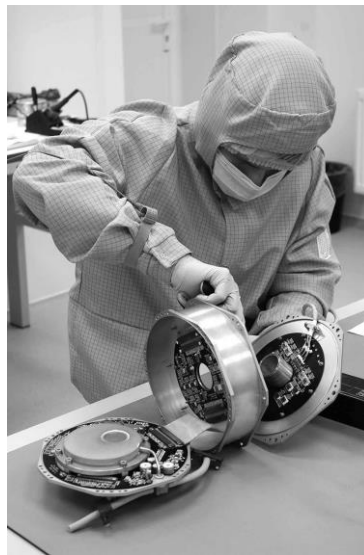
Figure 9. The top photo shows seven qualification-model (QM) DSSD CdTe crystals and their holders ready to assemble. The bottom images show the assembly process of the QM ART-XC X-ray detector blocks.
