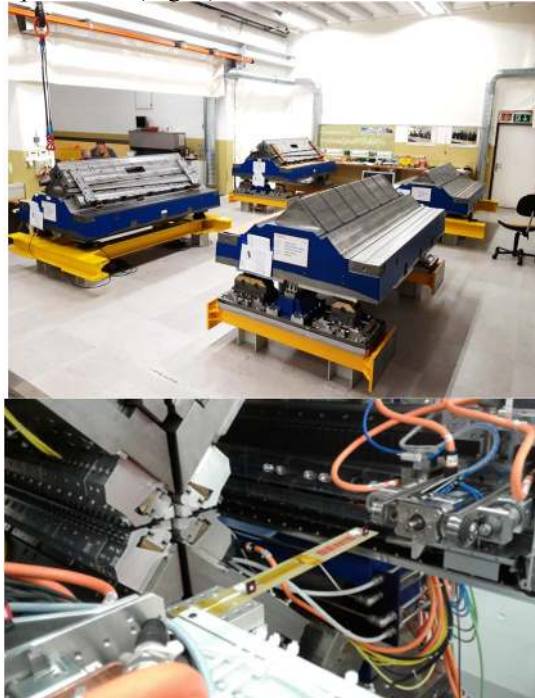
Figure 5: Assembly of the APPLE X undulator at the factory site (Top) and Hall probe measurements (bottom left) and motorized shimming screwdriver (bottom right).
