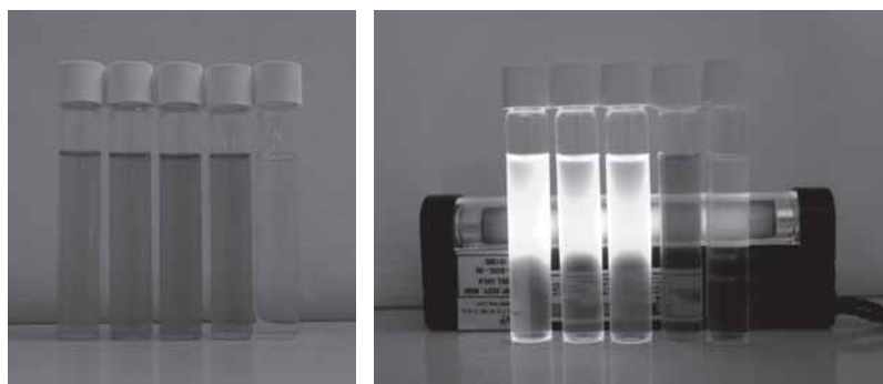
Fig. 2: Commercially available water test system. Out of five samples (tubes) four are positive for TC bacilli (left) and of those four, three are Esch. coli bacilli positive (right)
