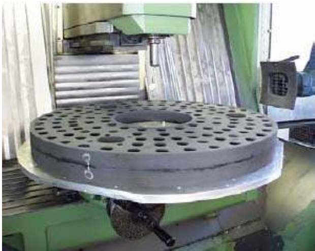
Fig. 5.2. Photos of numerically controlled milling being performed on carbon-carbon green-body material. Source: Ref. 44.
