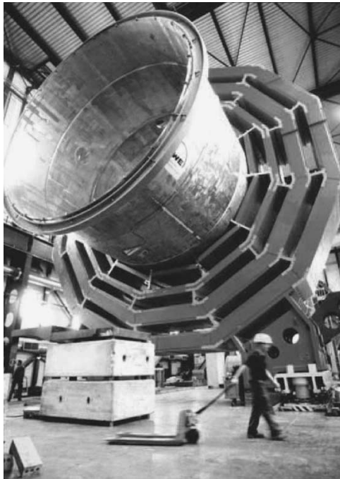
Fig. 2. View of the central barrel yoke ring equipped with the outer vacuum tank destined to house the superconducting coil.
