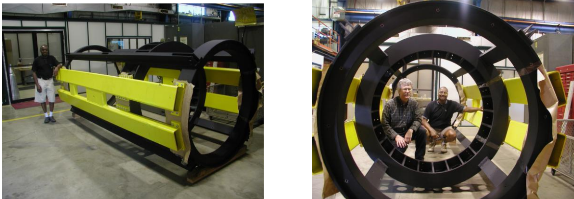
Figure 12 The DECam Cage(black) and lifting figure (yellow)
