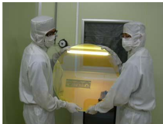
Figure 10 Asahi personnel hold a 620mm diameter glass substrate which has been coated with a short pass film (24 layers).
