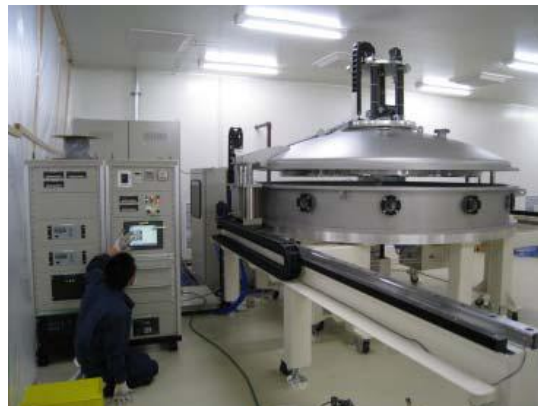
Figure 9 a) DES filter bandpasses achieved by Asahi on 100mm square filters b) Asahi engineer raises the cover of the ~3m diameter magnetron sputtering coating chamber that will be used for the DECam filters.
