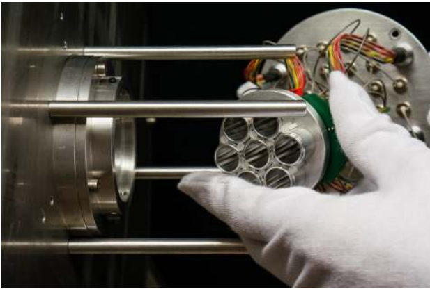
Fig. 3: Photo of the assembly of the FAMOUS SEVEN prototype focal plane with seven active pixels. The SiPMs (Hamamatsu-S10985-100C) are located behind the circular Winston cones.
