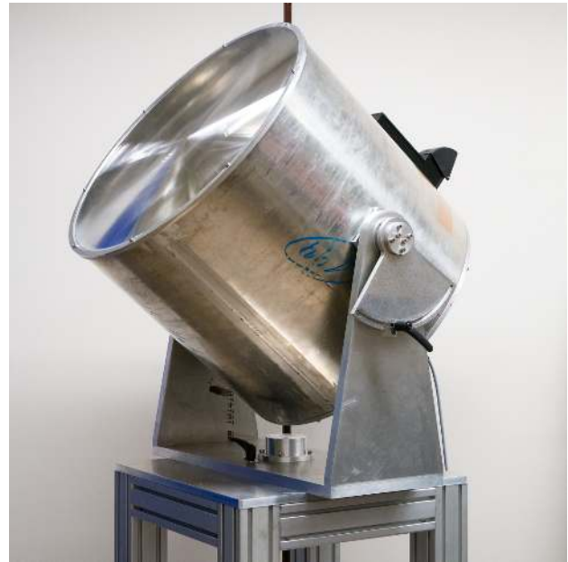
Fig. 4: Photo of the fully assembled FAMOUS SEVEN prototype with the Fresnel lens attached to the telescope tube which is fixed onto an altitude-azimuth mount.
