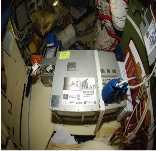
Fig. 13. Sci + WLS fiber + SiPM hodoscope system in space experiment LAZIO.
