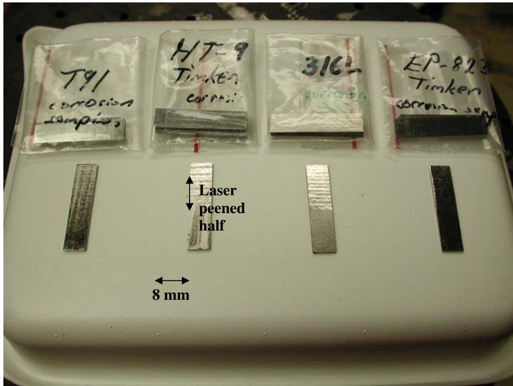
Figure 76. T91, HT-9, 316 L, and EP-823 Samples after Laser Peening.
