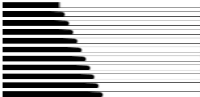
FIG. 11. Propagation of a chemical front in the presence of chemically induced Marangoni convection for M=-100 shown from top to bottom from t=0 up to t=50 with a time interval of \Delta t=5 . The aspect ratio between L_x=350 and L_z=10 is preserved.
