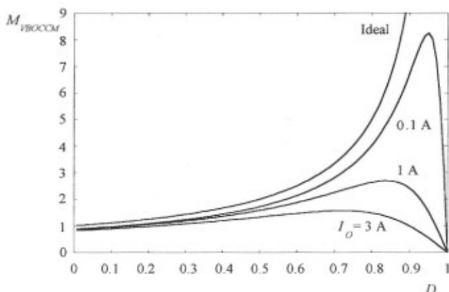
Figure 13. Voltage transfer function  $M_{VBOCCM}$  of a boost converter operated in the CCM, a constant output voltage  $V_O = 12$  V as a function of the duty cycle  $D$  with the DC output current  $I_O$  used as a parameter at  $f = 100$  Hz,  $R_{DS} = 55$  m $\Omega$ ,  $t_r = t_f = 100$  ns,  $V_F = 1.66$  V,  $R_F = 30$  m $\Omega$ ,  $L = 200$   $\mu$ H,  $R_L = 300$  m $\Omega$  and  $R_C = 20$  m $\Omega$ .
