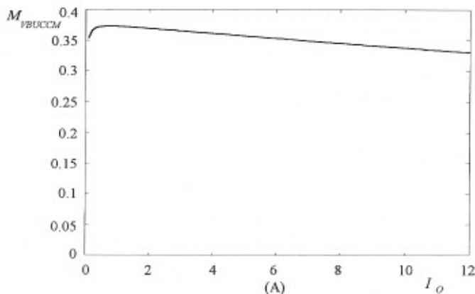
Figure 5. Voltage transfer function  $M_{VBUCCM}$  of a buck converter operated in the CCM, a constant output voltage  $V_O = 10$  V as a function of the DC output current  $I_O$  at  $f = 200$  kHz,  $R_{DS} = 55$  m $\Omega$ ,  $t_r = t_f = 80$  ns,  $V_F = 0.57$  V,  $R_F = 20$  m $\Omega$ ,  $L = 50$   $\mu$ H,  $R_L = 50$  m $\Omega$  and  $R_C = 50$  m $\Omega$ .
