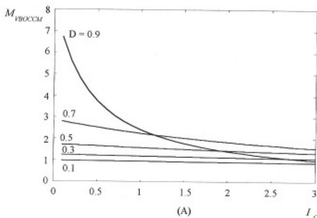
Figure 12. Voltage transfer function  $M_{VBOCCM}$  of a boost converter operated in the CCM, a constant output voltage  $V_O = 12$  V as a function of the DC output current  $I_O$  with the duty cycle  $D$  used as a parameter at  $f = 100$  kHz,  $R_{DS} = 55$  m $\Omega$ ,  $t_r = t_f = 100$  ns,  $V_F = 1.66$  V,  $R_F = 30$  m $\Omega$ ,  $L = 200$   $\mu$ H,  $R_L = 300$  m $\Omega$  and  $R_C = 20$  m $\Omega$ .
