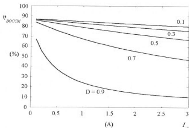
Figure 14. Efficiency  $\eta_{BOCCM}$  of a boost converter operated in the CCM, a constant output voltage  $V_O = 12$  V as a function of the DC output current  $I_O$  with the duty cycle  $D$  used as a parameter at  $f = 100$  kHz,  $R_{DS} = 55$  m $\Omega$ ,  $t_r = t_f = 100$  ns,  $V_F = 1.66$  V,  $R_F = 30$  m $\Omega$ ,  $L = 200$   $\mu$ H,  $R_L = 300$  m $\Omega$  and  $R_C = 20$  m $\Omega$ .
