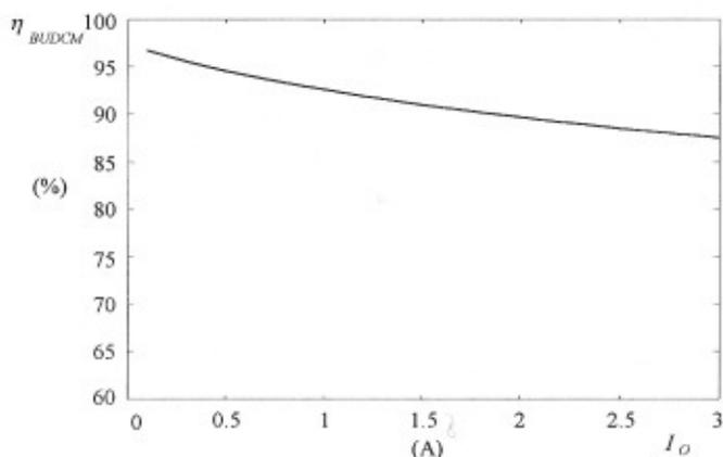
Figure 8. Efficiency  $\eta_{BUDCM}$  of a buck converter operated in the DCM, a constant input voltage  $V_1 = 28$  V as a function of the DC output current  $I_O$ , at  $f = 50$  kHz,  $R_{DS} = 55$  m $\Omega$ ,  $t_r = t_f = 80$  ns,  $V_F = 0.57$  V,  $R_F = 20$  m $\Omega$ ,  $L = 10$   $\mu$ H,  $R_L = 50$  m $\Omega$  and  $R_C = 50$  m $\Omega$ .
