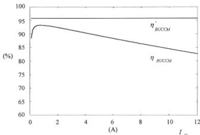
Figure 4. Efficiencies  $\eta'_{BUCCM}$  and  $\eta_{BUCCM}$  of a buck converter operated in the CCM, a constant output voltage  $V_O = 10$  V as a function of the DC output current  $I_O$  at  $f = 200$  kHz,  $R_{DS} = 55$  m $\Omega$ ,  $t_r = t_f = 80$  ns,  $V_F = 0.57$  V,  $R_F = 20$  m $\Omega$ ,  $L = 50$   $\mu$ H,  $R_L = 50$  m $\Omega$  and  $R_C = 50$  m $\Omega$ .
