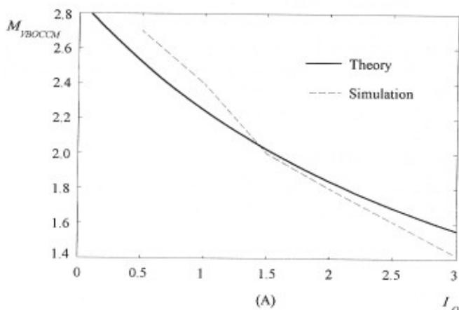
Figure 18. Voltage transfer function  $M_{V_{BOCCM}}$  of a boost converter operated in the CCM, a constant output voltage  $V_O=12$  V as a function of the DC output current  $I_O$  at a duty cycle  $D=0.7$  and a switching frequency  $f=100$  kHz.
