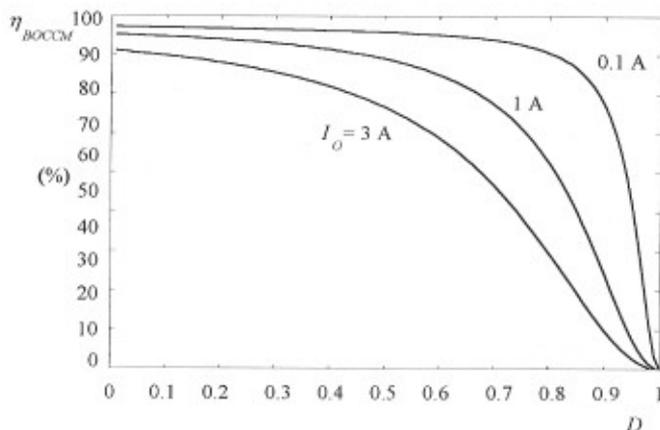
Figure 15. Efficiency  $\eta_{BOCCM}$  of a boost converter operated in the CCM, a constant output voltage  $V_O = 12$  V as a function of the duty cycle  $D$  with the DC output current  $I_O$  used as a parameter at  $f = 100$  kHz,  $R_{DS} = 55$  m $\Omega$ ,  $t_r = t_f = 100$  ns,  $V_F = 1.66$  V,  $R_F = 30$  m $\Omega$ ,  $L = 200$   $\mu$ H,  $R_L = 300$  m $\Omega$  and  $R_C = 20$  m $\Omega$ .
