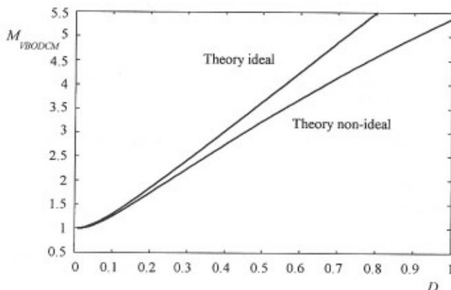
Figure 17. Voltage transfer function  $M_{V_{BODCM}}$  of a boost converter operated in the DCM, a constant output voltage  $V_O=48$  V as a function of the duty cycle  $D$  at  $I_O=0.65$  A,  $f=10$  kHz,  $R_{DS}=55$  m $\Omega$ ,  $t_r=t_f=150$  ns,  $V_F=0.57$  V,  $R_F=25$  m $\Omega$ ,  $L=10$   $\mu$ H,  $R_L=300$  m $\Omega$  and  $R_C=50$  m $\Omega$ .
