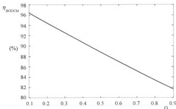
Figure 16. Efficiency  $\eta_{\text{BODCM}}$  of a boost converter operated in the DCM, a constant output voltage  $V_O = 48 \text{ V}$  as a function of the duty cycle  $D$  at  $I_O = 0.65 \text{ A}$ ,  $f = 10 \text{ kHz}$ ,  $R_{\text{DS}} = 55 \text{ m}\Omega$ ,  $t_r = t_f = 150 \text{ ns}$ ,  $V_F = 0.57 \text{ V}$ ,  $R_F = 25 \text{ m}\Omega$ ,  $L = 10 \mu\text{H}$ ,  $R_L = 300 \text{ m}\Omega$  and  $R_C = 50 \text{ m}\Omega$ .
