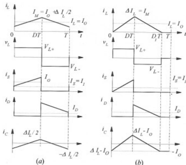
Figure 3. Steady-state current and voltage waveforms in a PWM buck converter. (a) continuous current mode; (b) discontinuous current mode.
