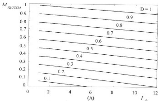
Figure 6. Voltage transfer function  $M_{VBUCCM}$  of a buck converter operated in the CCM, a constant input voltage  $V_I = 28$  V as a function of the DC output current  $I_O$  with the duty cycle  $D$  used as a parameter at  $f = 200$  kHz,  $R_{DS} = 55$  m $\Omega$ ,  $t_r = t_f = 80$  ns,  $V_F = 0.57$  V,  $R_F = 20$  m $\Omega$ ,  $L = 50$   $\mu$ H,  $R_L = 50$  m $\Omega$  and  $R_C = 50$  m $\Omega$ .
