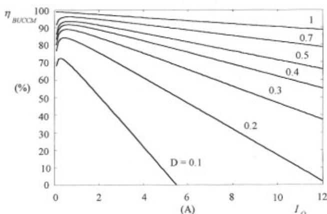
Figure 7. Efficiency  $\eta_{BUCCM}$  of a buck converter operated in the CCM, a constant input voltage  $V_1 = 28$  V as a function of the DC output current  $I_O$  with the duty cycle  $D$  used as a parameter at  $f = 200$  kHz,  $R_{DS} = 55$  m $\Omega$ ,  $t_r = t_f = 80$  ns,  $V_F = 0.57$  V,  $R_F = 20$  m $\Omega$ ,  $L = 50$   $\mu$ H,  $R_L = 50$  m $\Omega$  and  $R_C = 50$  m $\Omega$ .
