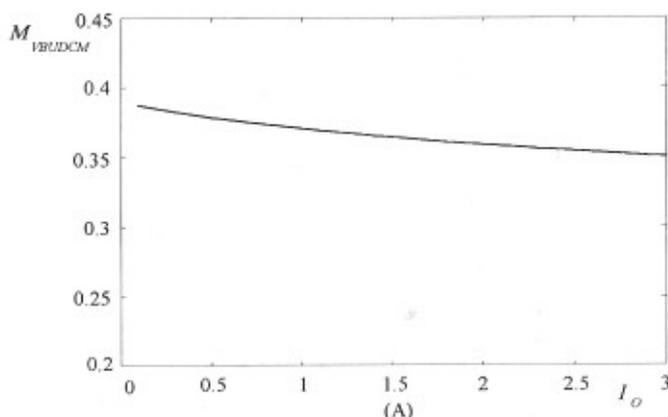
Figure 9. Voltage transfer function  $M_{VBUDCM}$  of a buck converter operated in the DCM, a constant input voltage  $V_1 = 28$  V as a function of the DC output current  $I_O$ ,  $f = 50$  kHz,  $R_{DS} = 55$  m $\Omega$ ,  $t_r = t_f = 80$  ns,  $V_F = 0.57$  V,  $R_F = 20$  m $\Omega$ ,  $L = 10$   $\mu$ H,  $R_L = 50$  m $\Omega$  and  $R_C = 50$  m $\Omega$ .
