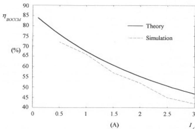
Figure 19. Efficiency  $\eta_{BOCCM}$  of a boost converter operated in the CCM, a constant output voltage  $V_O = 12$  V as a function of the DC output current  $I_O$  at a duty cycle  $D = 0.7$  and a switching frequency  $f = 100$  kHz.
