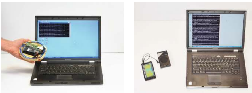
(a) Portable Instrument for Trace Acquisition (PITA), measuring the target and streaming the filtered signal over WiFi. (b) Experimental setup using a consumer AM radio receiver, placed near the target and recorded by a smartphone.
