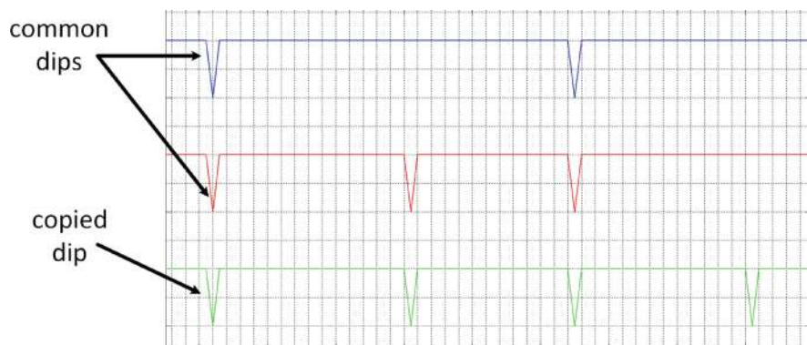
(b) After peak detection (the horizontal axis is the peak/dip number and the vertical axis is “high” for peaks and “low” for dips)
