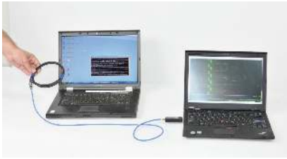
(a) A loop antenna (handheld) attacking a target laptop (left). The antenna is connected to an SDR receiver dongle attached to the attacker’s computer (right).
