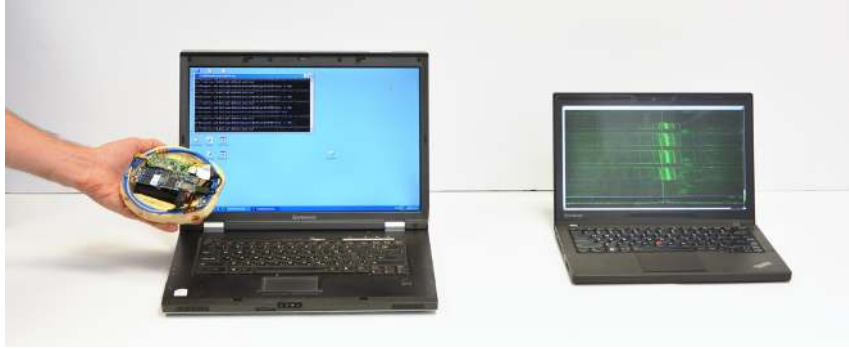
Figure 11: Untethered measurement device in online mode. The PITA (handheld) measures the target computer (left) at a specific frequency band and streams the digitized signal over WiFi, in real time, to the attacker’s computer (right). The attacker’s computer can be many meters away when using a direct WiFi connection, or (if the PITA is configured to use a suitable WiFi access point) anywhere on the Internet.
