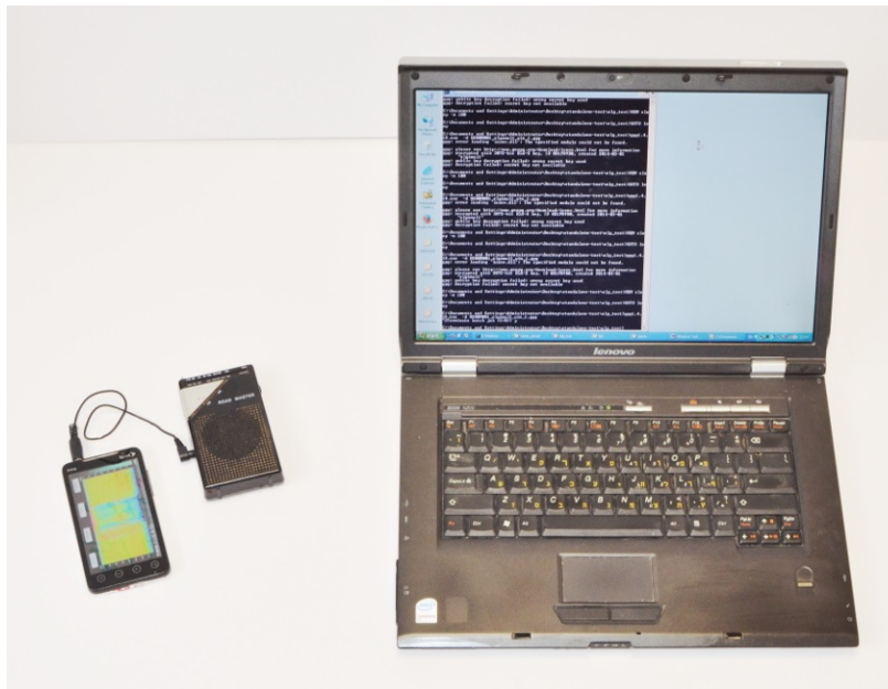
Figure 13: The radio-based experimental setup attacking the Lenovo 3000 N200 target. The radio receiver is placed near the target and tuned to approximately 1.5 MHz. The radio's output is connected, through the adapter cable, to the input of an HTC EVO 4G smartphone recording at 48 Ksample/sec.
