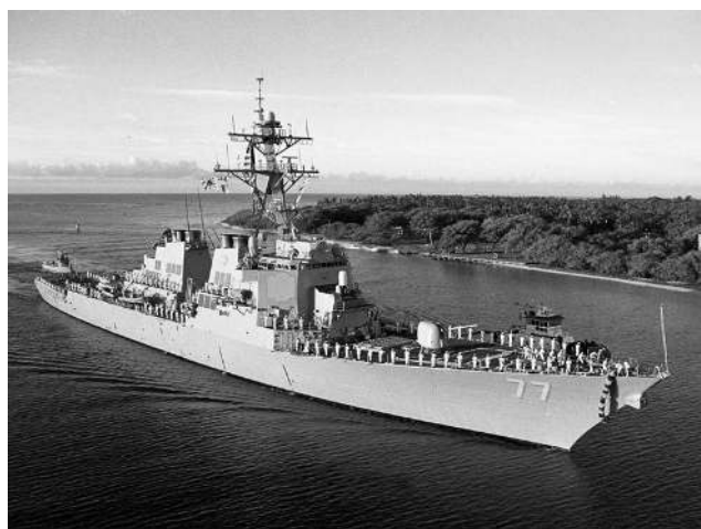
Figure 1: The O'KANE (DDG 77) is an Arleigh Burke (DDG 51)-class guided-missile destroyer, 505 feet long, with a 59-foot beam, and a displacement of 8,400 tons. Powered by four LM2500 gas-turbine engines that can generate more than 100,000 shaft horsepower, her top speed exceeds 30 knots.
