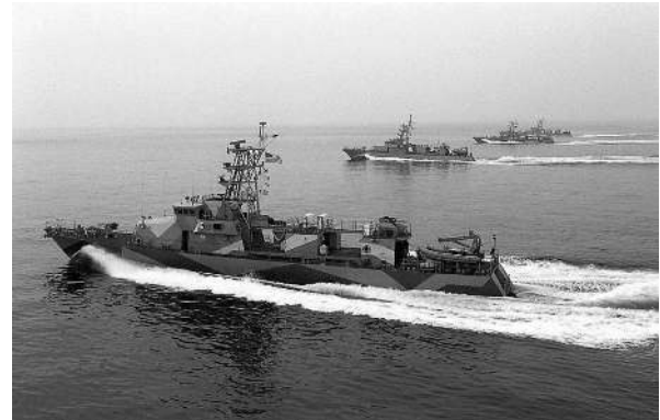
Figure 4: PC 1-class Patrol Coastal ship HURRICANE displaces 331 tons, is 170 feet long, with a beam of 25 feet, and is powered by four diesel engines, each with its own shaft and screw.
