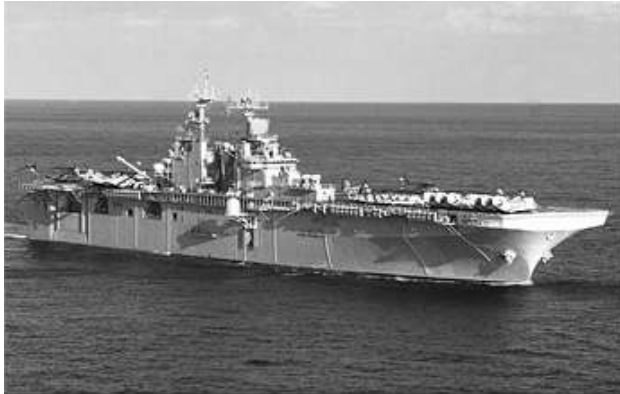
Figure 6: The Amphibious Assault Ship USS WASP (LHD 1) is 844 feet long, with a beam of 106 feet. Two steam boilers and two shafts that generate 70,000-shaft horsepower power this 40,650-ton ship. Source. Department of Defense.
