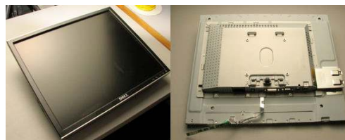
Figure 5. Starting stages: the original monitor (left), and with case removed (right)
