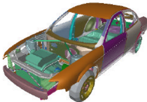
Figure 2. ULSAB Vehicle Crash Model.
