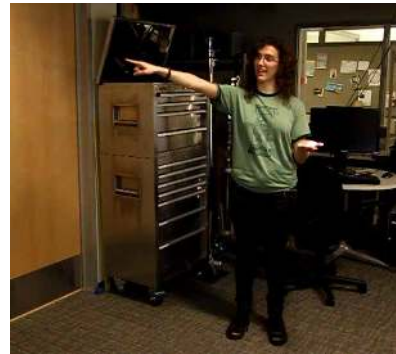
Figure 6. Master and Commander allows the user to take projected graphics from the wall into their hand and then place the objects on another part of the room. Here the user is holding a graphic in their left hand while pointing at a destination. Saying “put that there” will cause Beamatron to animate the object to the wall, where it will find a surface to “hang” the graphic.
