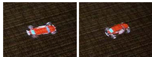
Figure 3. Beamatron rendering pipeline corrects projected graphics to account for projection surface distance and shape. This can be used to correctly project graphics for a particular viewpoint. Left: projective texturing disabled—the car is rendered from the projector’s viewpoint. Right: projective texturing enabled—the car is rendered for the user’s view.
