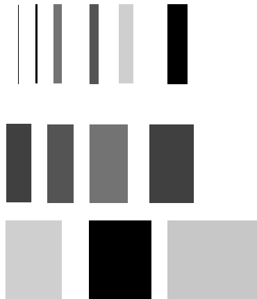
Figure 4-6: Schematic illustration of image model used to analyze expected phase-energy histogram characteristics. We assume an image consists of rectangles of a wide range of sizes and contrasts.
