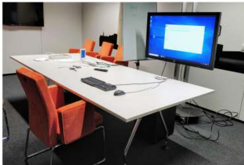
Fig. 13. The setup used for the subjective experiments showing the 1080p Barco LC-47 monitor at eye-height. Both the ground truth and compressed sequences were shown side-by-side at native resolution.
