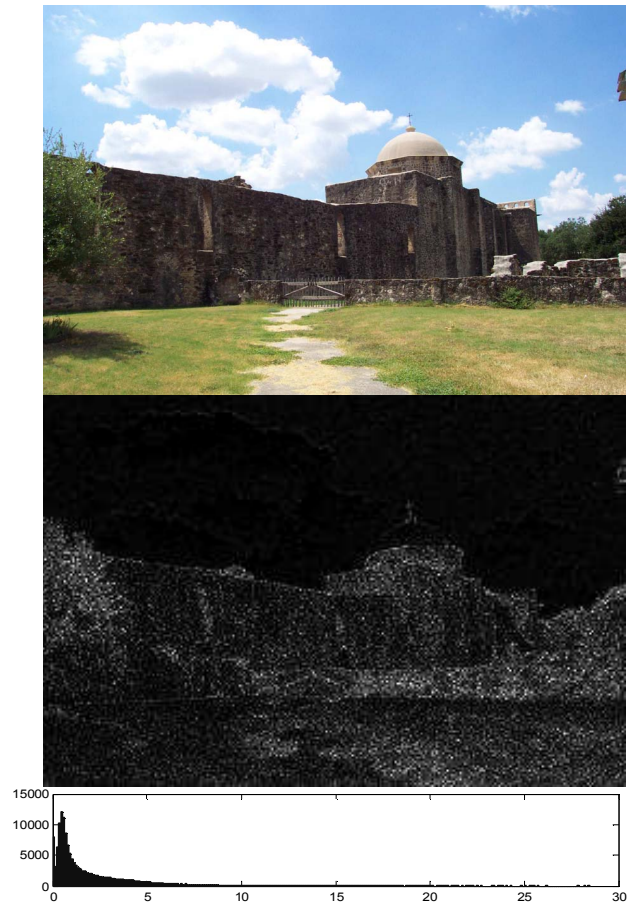
Figure 5 Top: Original image, Middle: noise variance estimate in 8x8 pixel blocks. Bottom: Histogram of the noise variance estimated for each 8x8 block.
