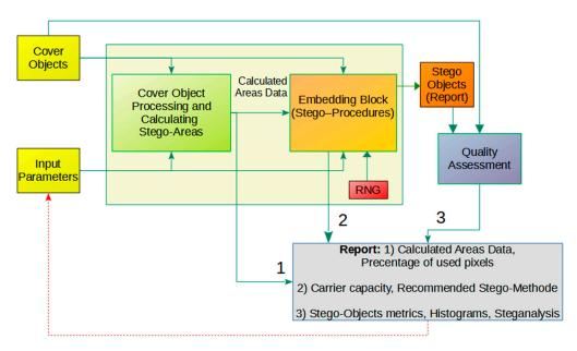
**Figure 1.** The block diagram of the system.
