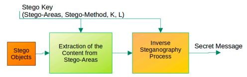
Figure 8. Block diagram of extraction procedure.
