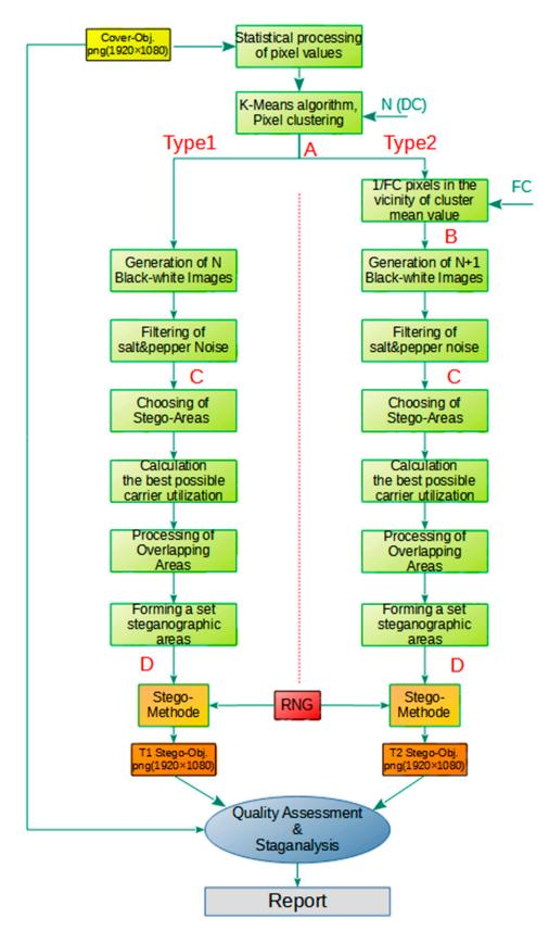
Figure 2. Detailed System Block Diagram.
