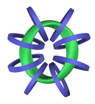
FIG. 1: Magnetic-field coils and plasma boundary for ES-TELL, a two-period quasisymmetric stellarator [6]. The 8 coils are all identical and circular.
