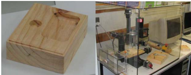
Figure 12 Sampled machined part and CNC milling machine (see online version for colours)
