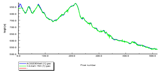
Figure 7: Comparison of a profile in PRISM DSM (green) and reference DTM (blue) in the northern part of the images. The profile is along-track.
