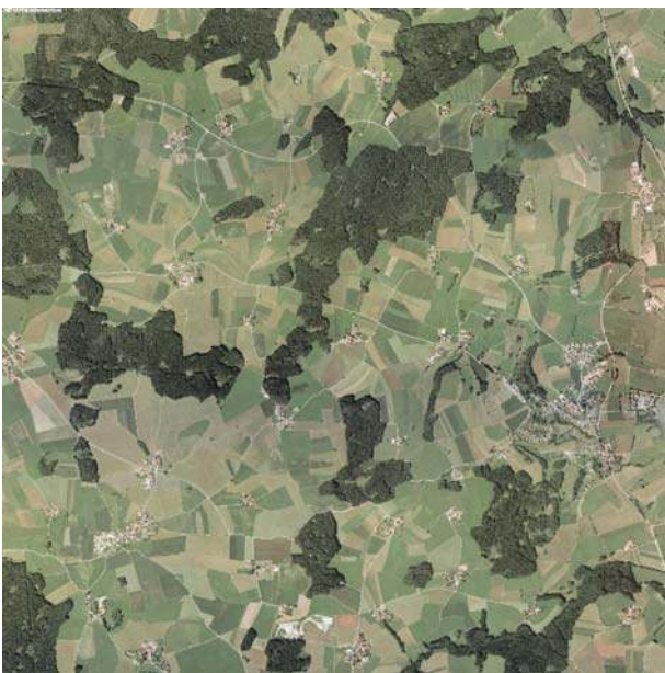
Figure 5: Orthoimage of Taching area from Bavarian Survey as a source for GCP (2 m sampling)
