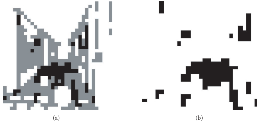
FIGURE 3: (a) The initial occlusion field as it has been formed after a two-threshold-level classification. The grey colour indicates the uncertain blocks, whereas the black colour indicates the occluded blocks. (b) The final occlusion field after the occlusion phase of the energy minimization process. The occluded region has been augmented because the employed algorithm favours occlusion connectivity.
