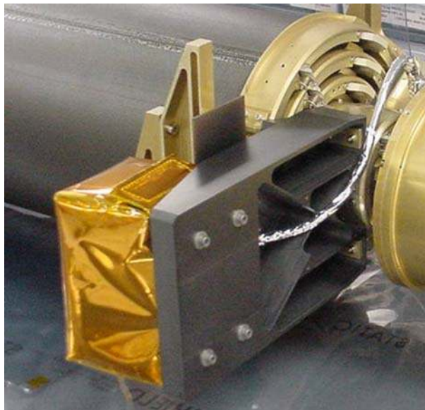
Fig. 13 Photograph of an IMPACT MAG flight unit on its boom tray
