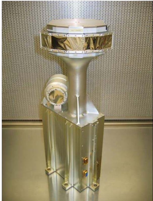
Fig. 16 Photograph of a LET and HET flight unit, together with a SEP Central box. LET has the wide-field telescope head at the top of the picture. HET is the smaller cylindrical telescope in the middle left of the LET platform column
