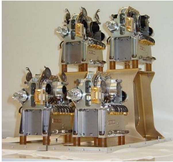
Fig. 14 Photograph of the SEPT telescope pairs (SEPT-E and SEPT-NS) for both spacecraft, showing their aperture doors open on the left , and closed on the right
