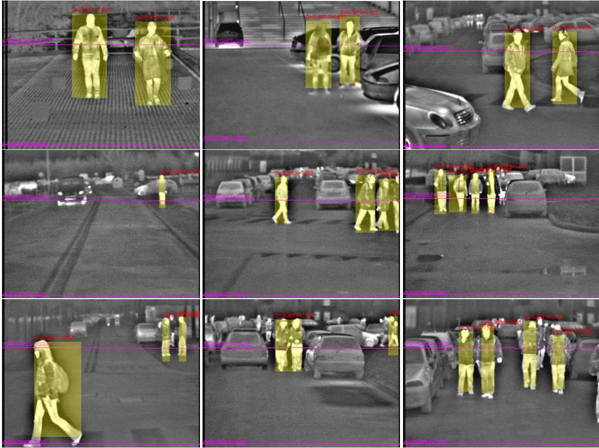
Figure 7: Pedestrian detection results: detected pedestrians are showed using a superimposed yellow box. Each box also shows the distance and height of detected object. The two magenta lines show the minimum and maximum distances used for the detection.
