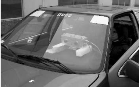
Fig. 1 The sensor of I.N.S.A. installed into ARGO.
