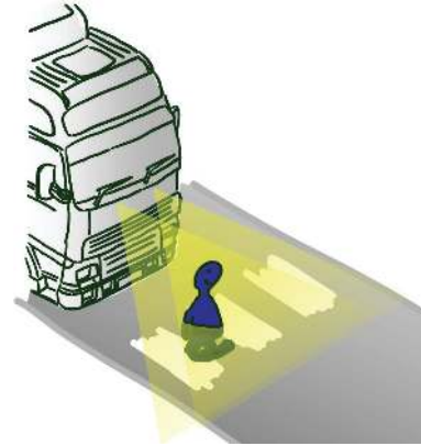
FIGURE 3: Start-inhibit protection system.
