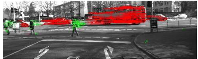
(b) Feature tracking (5 frames, static camera)
