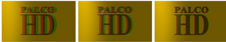
Figure 3 Effect with anaglyph examples of parallax variation in sequence Palco HD.
