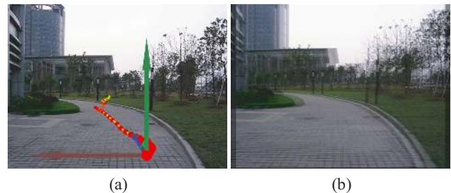
Fig. 10. A poor example of stereoscopic video generation. The input monocular sequence is taken by a hand-held camera moving in the direction of the camera viewing direction. (a) shows the recovered base trajectory. Since the angle between the moving direction and the viewing direction is very small, the binocular parallax is hard to be converted from the motion parallax. As the result, all binocular parallax of the sample points in the scene are almost identical, and the generated stereoscopic video does not properly show the depth cue.
