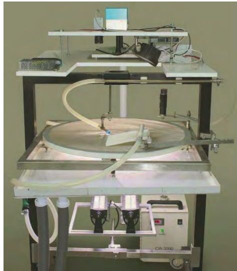
Figure 3. Upper drawing: Camera set-up for sorting male and female Aedes pupae based on size dimorphism. (Drawing from Zacarés et al. 2018, reproduced with permission.) Lower photo: Prototype laser sex-sorting machine (Bourtzis 2019).
