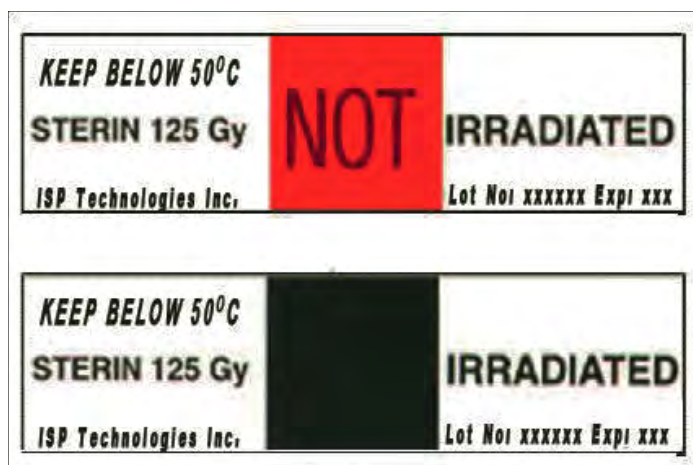
Figure 5. Radiation-sensitive indicators before (upper) and after (lower) exposure at dose >125Gy (© ISP 2002). (Figure from FAO/IAEA/USDA 2019.)
