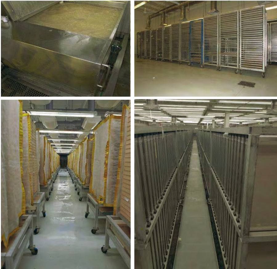
Figure 2. Mass-rearing the Mediterranean fruit fly at the El Pino facility, Guatemala. Upper left: Eggs treated in a hot-water bath to kill female embryos of the temperature-sensitive lethal sexing strain; Lower left: Rearing larvae in trays, showing hanging plastic net sheets to redirect jumping mature larvae to the collection pan below; Upper right: Maturing pupae in trays stacked on trolleys; Lower right: Vertical cages for adult emergence, feeding, and egg oviposition and collection. (Photos from C. Cáceres, reproduced with permission.)
