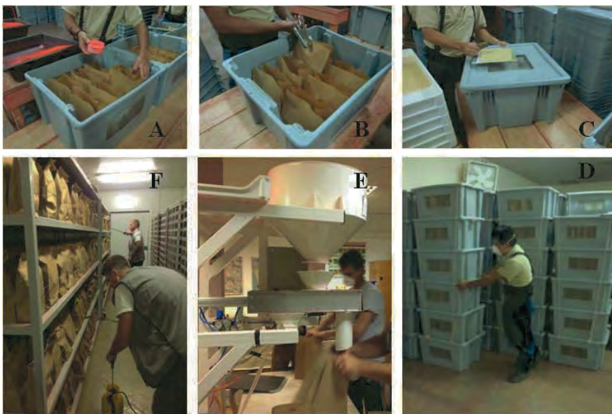
Figure 2. Mediterranean fruit fly emergence and release facility in Retalhuleu, Guatemala, showing clockwise: A: Worker placing sterilized dyed pupae into a PARC emergence box; B: Stapling paper bags in the centre to permit flies to leave the bag; C: Placing one modified agar-block diet; D: Stacks of six PARC boxes inside an adult emergence room. At the Neretva Valley, Croatia, Mediterranean fruit fly programme: E: Machine for loading pupae into paper bags; F: Adult emergence room containing bags for fly emergence. Water is provided/sprayed through the surface of the bag.
