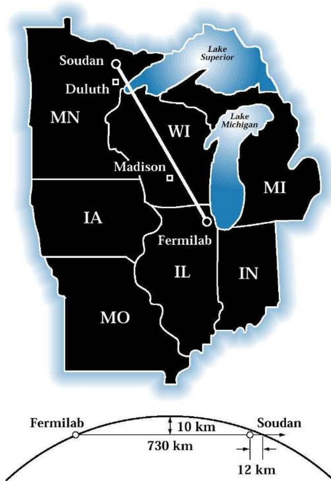
Figure 3.1: The MINOS neutrino beamline. The \nu_\mu/\bar{\nu}_\mu beam is produced in the NuMI facility at Fermilab. It passes through the ND at Fermilab and the FD in the Soudan mine in northern Minnesota. The baseline is 735 km. The figure is taken from Reference [73].
